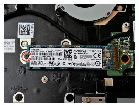
Remove the single 3.6 mm screw holding the left side of the M.2 SSD card with a Phillips PH0 screwdriver.
