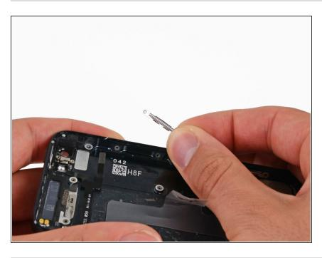
Remove the four front panel clips from the rear case.
