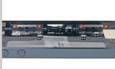
Remove eight 1.3 mm Phillips screws securing the front panel clips to the interior sides of the rear case.
