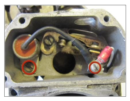
Locate the two screws on the back of the magneto that holds the capacitor in place.
