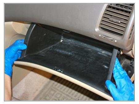
The glove box is held in place by tabs on both sides. Push inward on both sides of the box to allow the glove box to drop clear the tabs and drop downward slowly.
