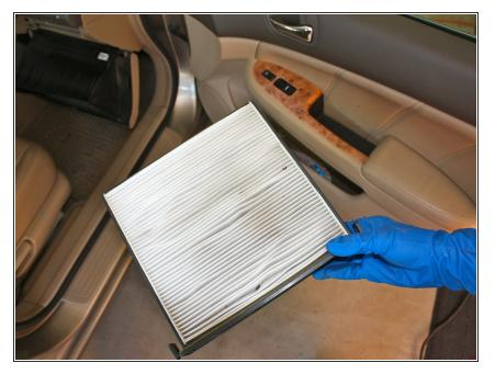
Push the air filter out of the plastic housing from the bottom and discard.
