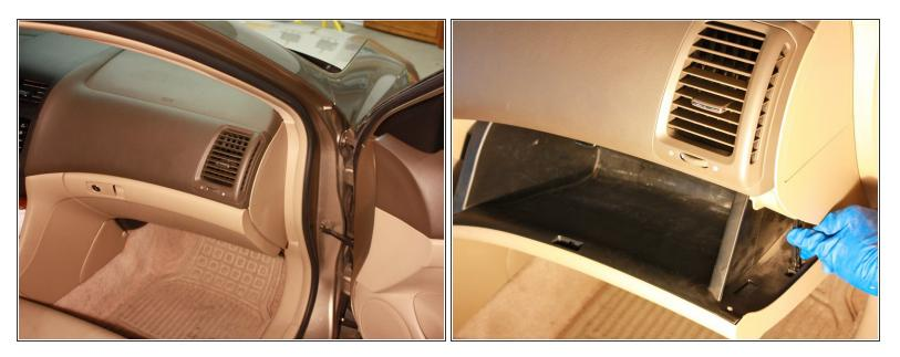
• Open the passenger side door and locate the glove box. Open and empty the glove box.
