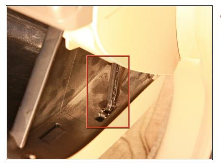
Identify the glove box damper assy latch on the right side of the glove box. Using moderate force, press against the latch with your thumb until it pops out of place.
