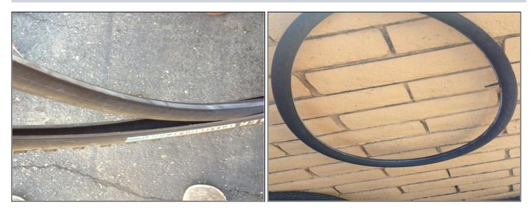
• Remove the inner tube from the tire by simply pulling it from the tire carcass.
