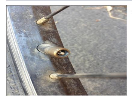
Locate the valve stem and remove the valve stem cap if one is present.
