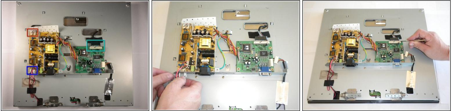
**⚠** Use caution when removing the connectors as they can easily break when removing.
