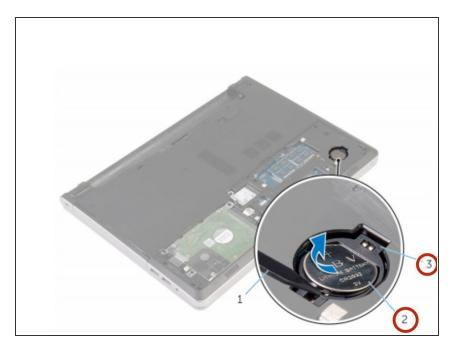
Using a plastic spudger, gently pry the coin-cell battery out of the battery socket on the system board.
