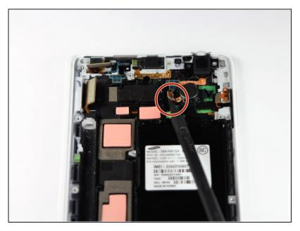
Insert the sharp end of the spudger underneath the golden cables connecting the vibration motor. Gently pry upwards to disconnect them.
