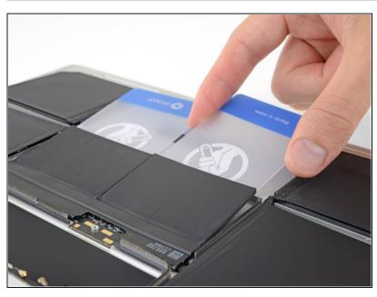
• Repeat the previous step to separate the final battery cell.
