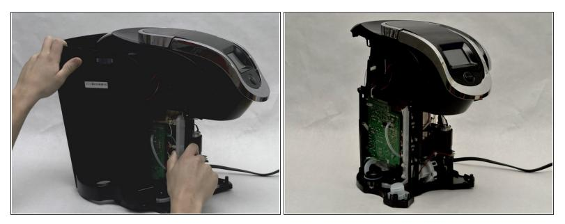
Remove the entire back exterior surrounding the Keurig by removing the latches connecting the back exterior to the silver frame on top. To do this, use the metal spudger to lift the latches up and out.
