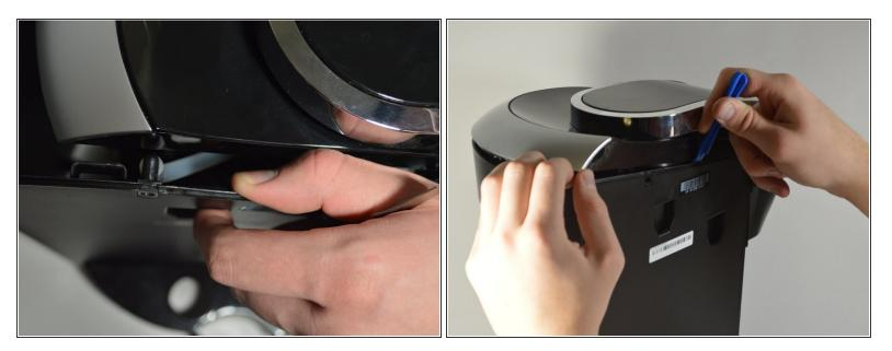
Separate the side panel from the top frame of the brewer, using the blue opening tool for help if necessary.
