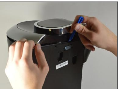
Separate the side panel from the top frame of the brewer, using the blue opening tool for help if necessary.
