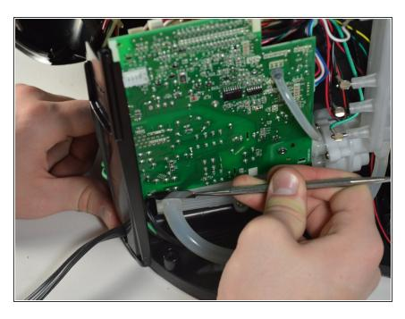
Using the metal spudger, snap the circuit board out of the latches on the bottom of the board.
