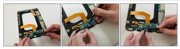
• Flip the motherboard over and locate the ribbon attaching the Rear Camera to the motherboard. Carefully pop off the ribbon from the logic board with the flat end of the **spudger**.
