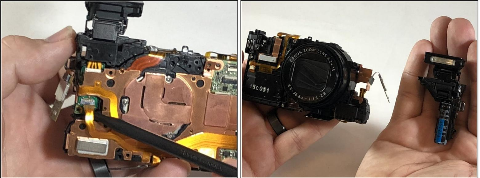
**!** Flash contains charged capacitor. Shock hazard.
