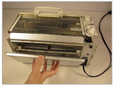
• Remove the crumb tray (the bottom, metal panel) from the toaster unit.
