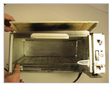
• Finish removing the outside cover by lifting the lid upward.
