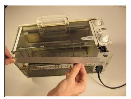
• Remove the aluminum strip from the bottom of unit; this is the piece that is directly under the door.
