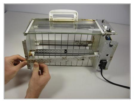
Remove the the heating coil protection bar from the toaster unit by first pulling out the left side.
