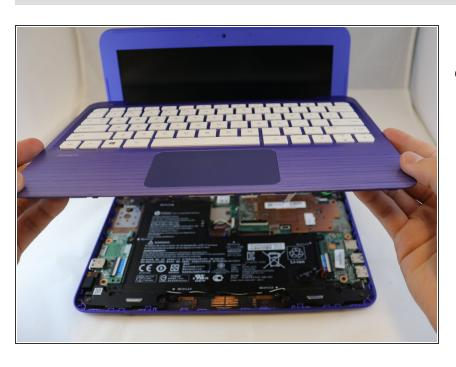
After detaching the two large ribbon cables, carefully lean the keyboard against the screen.
