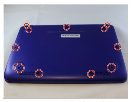
Using the Phillips #1 screwdriver, remove all 11 of the the 5mm screws.
