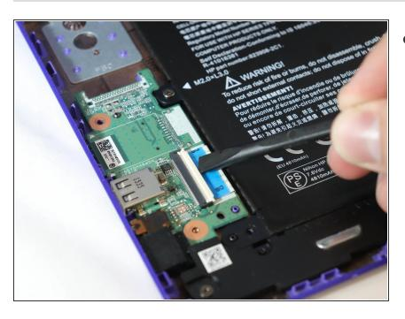
Use the black nylon spudger to flip the tab up that holds the ribbon cable in place.
