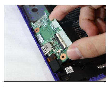
Lift the USB port out and remove it from the device.
