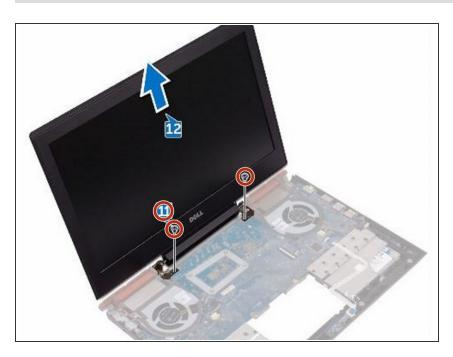
Replace the two screws (M2.5x5) that secure the display assembly to the computer base.
