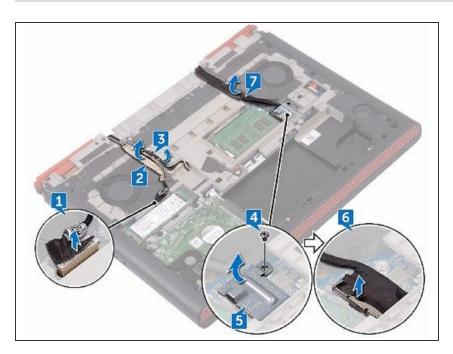
• Route the antenna cables through the routing guides on the computer base.
