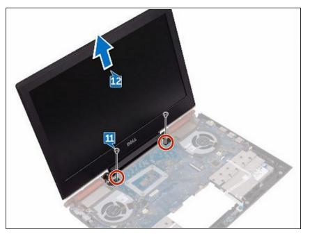
Align the screw holes on the NEW display assembly with the screw holes on the computer base.
