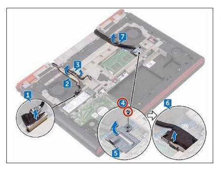
Replace the screw (M2x3) that secures the display cable bracket to the system board.
