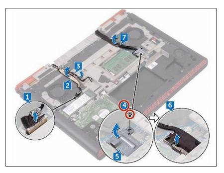
Remove the screw (M2x3) that secures the display-cable bracket to the system board.
