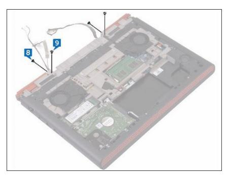
Remove the two screws (M2.5x5) that secure the display assembly to the computer base.
