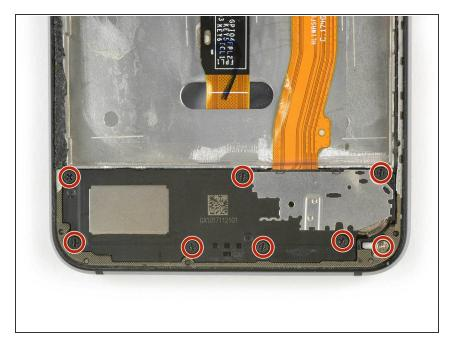
Remove the eight Phillips #00 screws securing the loudspeaker.
