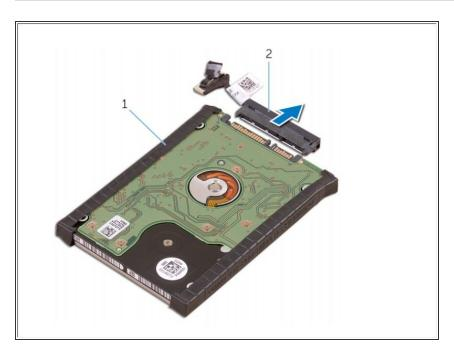
Disconnect the hard drive interposer from the hard drive assembly and then remove the hard drive covers away from the hard drive.
