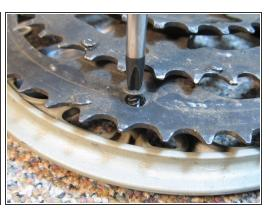
Use a Phillips #2 screwdriver to remove the four screws on the back of the chainring.
