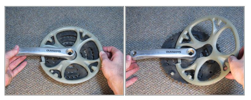
Hold on to the crank arm and pull out the chain guard gently.
