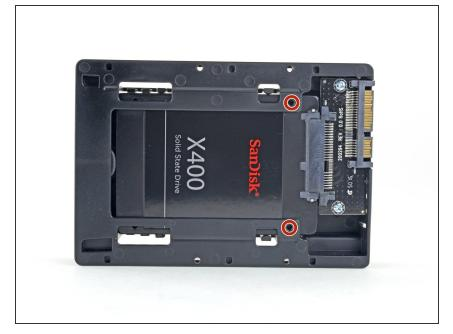
You may optionally install two Philips #1 screws that came with the enclosure kit to secure the SSD in the enclosure.
