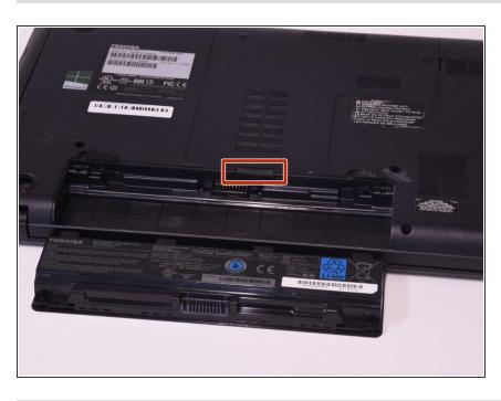
Holding the left tab in place, use the groove located between the two tabs to pry the battery up and out.
