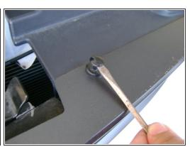
Remove all the pins on the front cover to gain access to the back of the grille.
