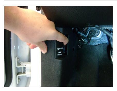
Pull the latch by the drivers feet to open the hood.
