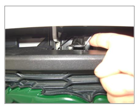
Push the latch under the center of the car's hood.
