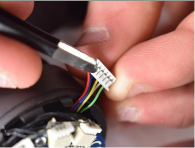
• Pull out the white wire connecter that is currently in the wire assembly.
