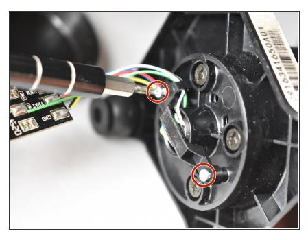
Using the Philips #000 screwdriver, unscrew the two 5.9 mm screws and remove the retaining clip on top of the motor piece.
