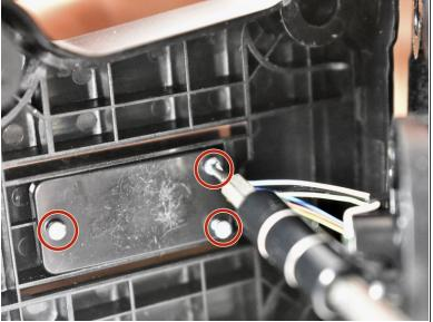
Prop the top cover of the motor piece off the Motor Battery Component. Using Phillips #00 screwdriver, unscrew the three screws (their lengths are 5.9 mm) that are in this top cover piece.
