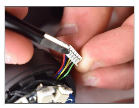
Remove the white wire connector cap using the tweezers. This is for the wires that are currently in the motor piece. Do take note of the orientation and order of the wires.
