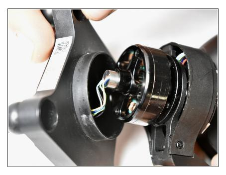
Once these screws are removed, pop off the top of the motor piece.
