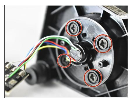
Using the Phillips #1 screwdriver, remove the four 6.3 mm motor mount screws on top of the motor piece.
