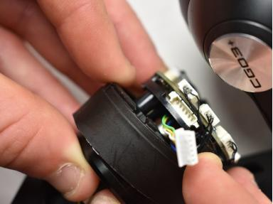
Removed the damaged slip ring motor by guiding the wires through the opening in the motor piece.
