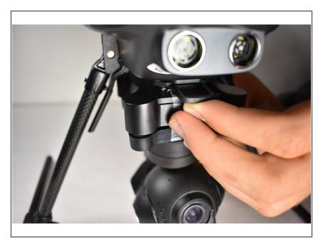
Remove the Motor Battery
