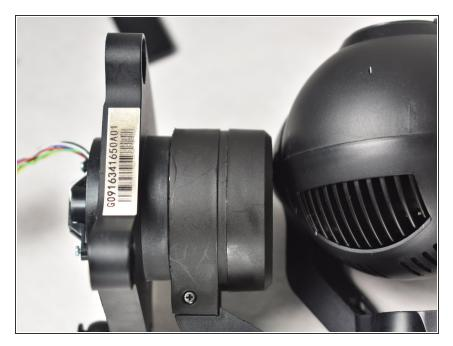
Grabbing the Motor Piece, remove the bottom cap of this motor piece.
