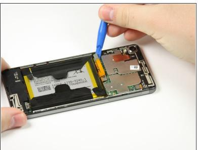
Pry up the copper connector next to the battery with the plastic opening tool.
