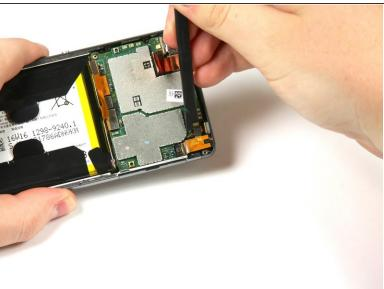
• Use the spudger to loosen the black connector from the top right of the motherboard.
