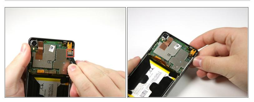
Use the spudger to take off the connector in the top right of the motherboard.
