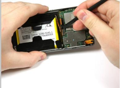
• Use the spudger to detach the three copper connectors on the bottom area of the motherboard.
