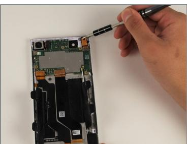
• Remove the 4mm T5 screw connecting the headphone jack to the panel.
