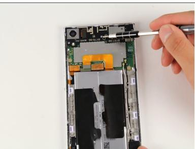
Remove the four 4mm T5 screws on the top of the black panel securing the antenna module to the device.
