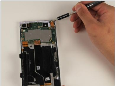
Remove the 4mm T5 screw connecting the headphone jack to the panel.
