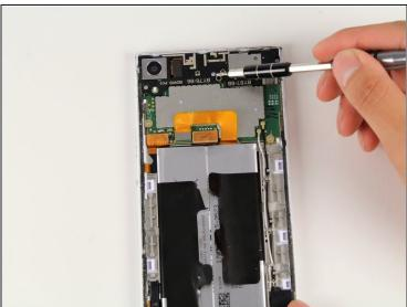
• Remove the four 4mm T5 screws on the top of the black panel securing the antenna module to the device.
