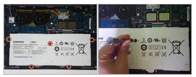
• Remove the five 4.3mm Phillips #00 screws from the battery.
