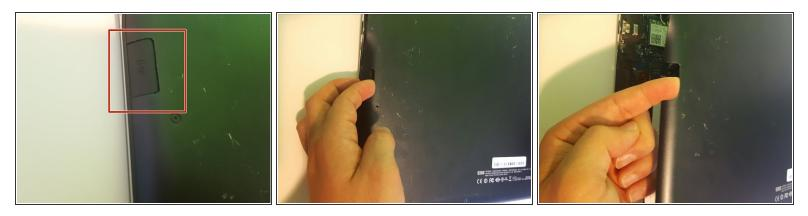
• Press the button to release the bottom cover.
