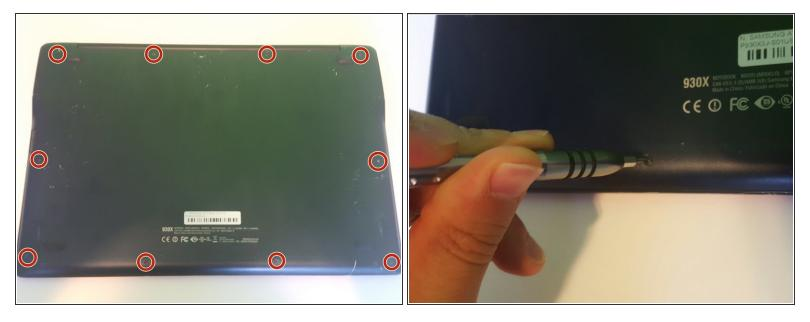
• Remove the ten 4.3mm Phillips #00 screws from the bottom cover of the laptop.
