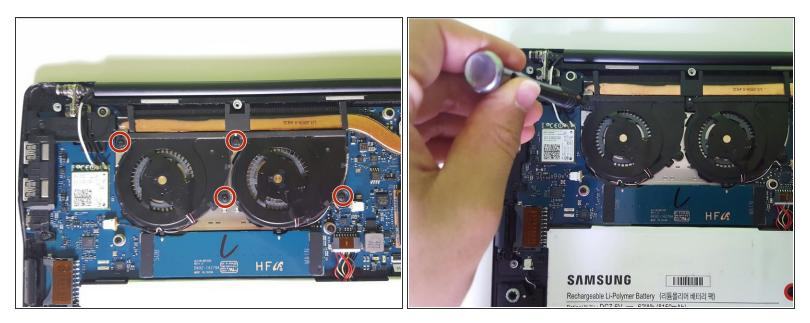
• Remove the four 4mm Phillips #00 screws from the fans.
