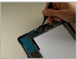
Using the tweezers, remove the green protective film from the connector between the rear camera and the motherboard.
