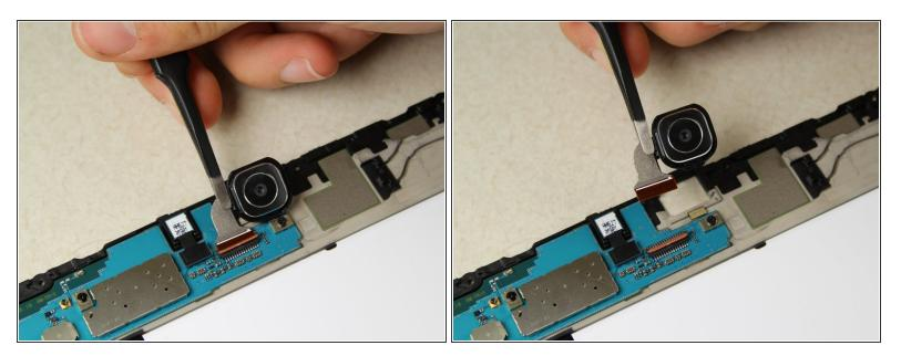
Pull the connector out of the slot using tweezers and remove the camera.
