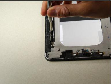
Remove the 2 centrally-located black 3.0 mm Phillips head screws using the screwdriver.
