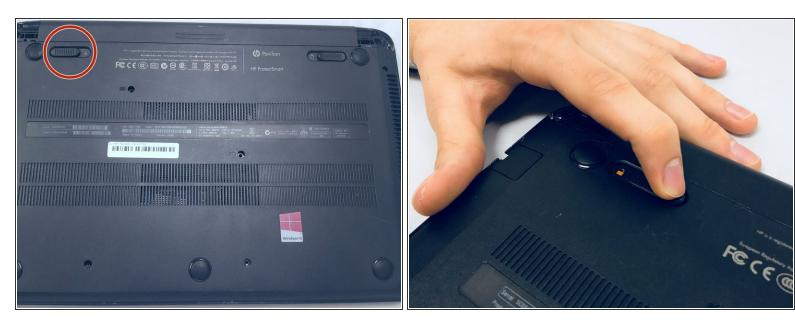
Flip the computer over and move the battery lock switch to the "unlocked" position (marked by an orange lock icon).
