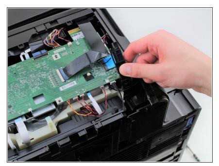
Remove the black brace from the right side of the motherboard, located near the black ribbon cable.
