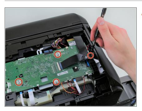
Remove the four 6.5 mm T10 Torx screws from the motherboard.
