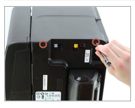
Remove the two 12mm T10 Torx screws on the top edge of the printer.
