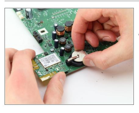
Remove the battery by grabbing its edges, lifting upward, and sliding sideways. To reassemble your device, follow these instructions in reverse order.
