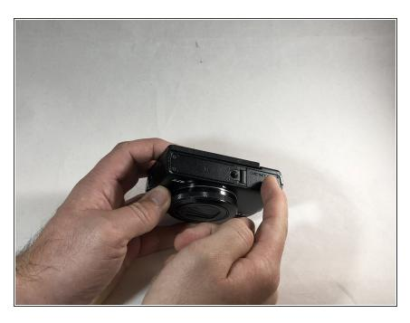
Slide the cover latch towards the center of the camera using your finger.
