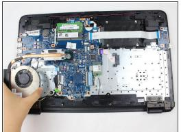
Once the fan is unplugged from the motherboard, remove the 6 mm screws with a Phillips #1 screwdriver that are connecting the fan to the laptop. Remove the fan.
