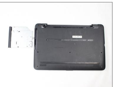
Once the screws are removed, carefully remove the CD player port.
