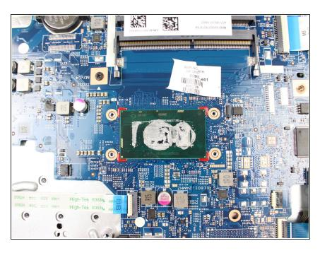
Once the fan is removed, you will see the hot plate that transfers the heat from the laptop to the fan. You will need to add thermal paste to the hot plate before placing your replacement fan back on.
