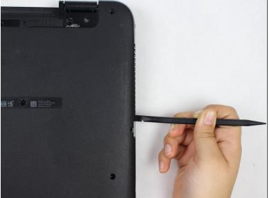
Once you have removed the CD player port, use the spudger tool to carefully remove the back panel.
