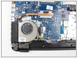
To remove the fan, start by unplugging the fan from the motherboard.
