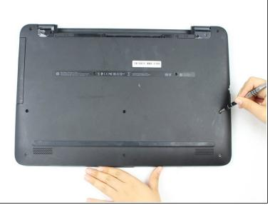
Remove the fourteen 8 mm screws with the Phillips #1 screwdriver.
