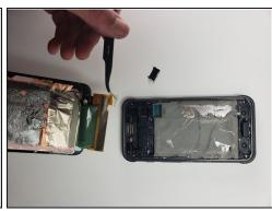
• Use the <u>tweezers</u> to disconnect the screen from the phone by detaching the connection.
