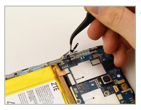
Use the tweezers to pull back on the cable connecting the power and volume button until it is removed.
