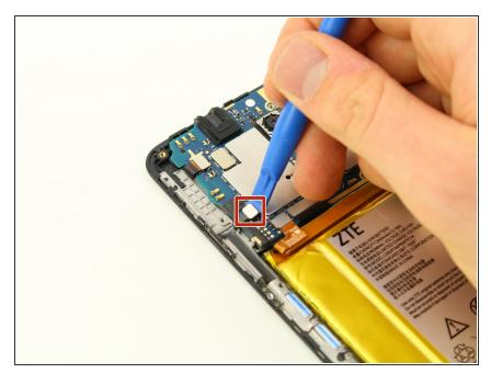
Use the plastic opening tool to remove the lower left connector on the motherboard.
