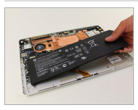
Lift the battery out of the device.
