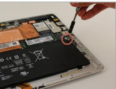
Remove all six Phillips 3 mm screws around the battery by rotating in the counterclockwise direction with a Phillips screwdriver.
