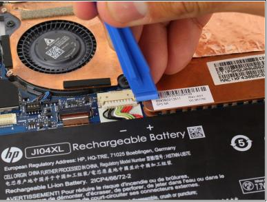
Remove the battery's connector by pushing both sides of the tab towards yourself with a plastic opening tool.
