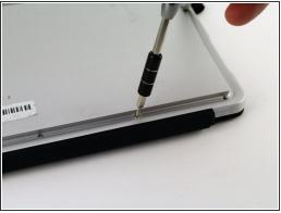
Remove the six 3mm Torx T5 screws underneath the kickstand.
