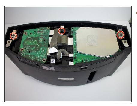
Remove the three 15.5mm PH2 screws holding the front-mesh grille in place.
