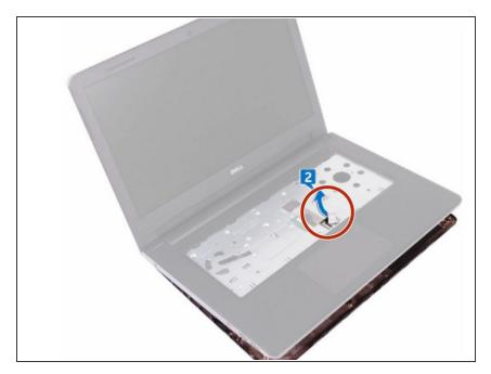
Place the base cover on the palmrest assembly and route the opticaldrive cable through the slot on the palm-rest assembly.
