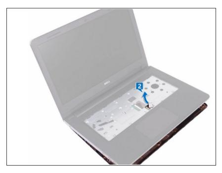
Slide the optical-drive interposer into the tabs on the **NEW** base cover and snap it into place.
