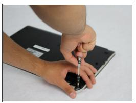
Remove all 14 of the 4 mm screws on the back side of the laptop with a Phillips #1 screwdriver.
