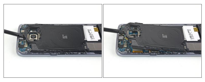
• Use the flat end of a spudger to lift the charging coil assembly out of the phone.
