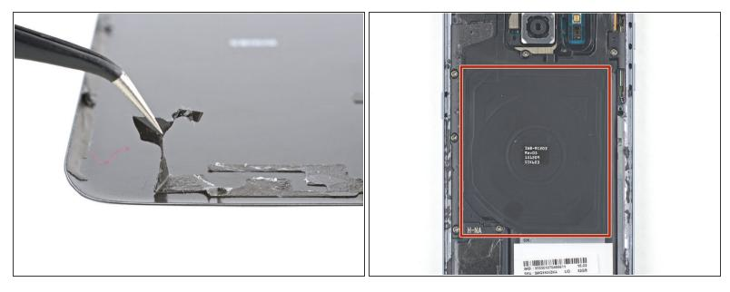
To reinstall the back cover with a custom-cut adhesive strip, follow this guide.
