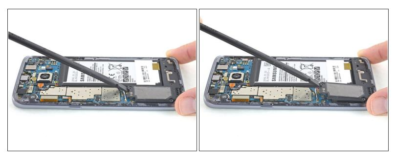
Use the flat end of a spudger to pry up and remove the loudspeaker assembly.
