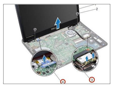
Make a note of the cable routing and disconnect the display cable and the wireless card antenna cables from the connectors on the Mini-Card.
