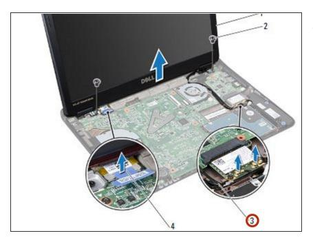
Make a note of the routing of the Mini-Card antenna cables and the display cables. Remove the cables from the routing guides.
