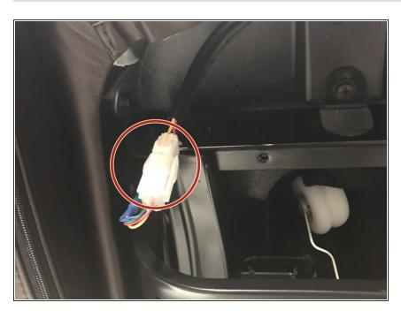
this speaker wire at the top left of the frame will need to be disconnected.
