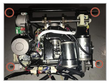
The new mech will not come with the plastic wheels, these will need to be transferred from the old mech to the new one. see photo for location of wheels.
