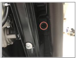
• Remove all 6 screws on frame. 2 up top and 2 on both sides.
