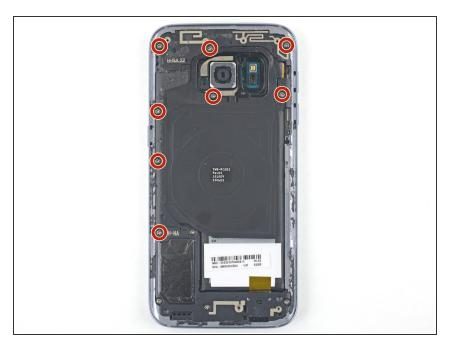
Remove the eight 3.5 mm Phillips screws securing the NFC antenna and charging coil assembly.
