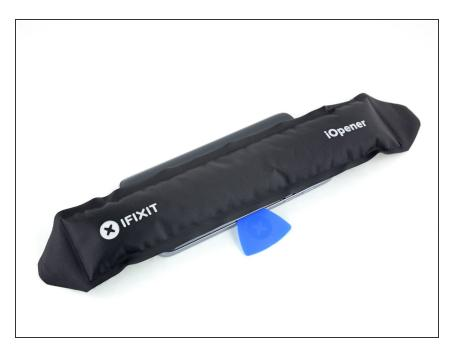
Once you have the pick firmly inserted into the glass, reheat and reapply the iOpener to soften the adhesive.
