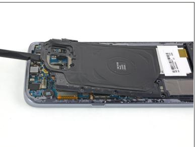
Use the flat end of a spudger to lift the charging coil assembly out of the phone.
