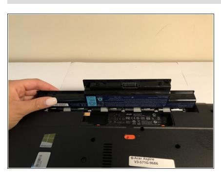
While holding the lever to the right, use your fingers to lift the battery up and out of the compartment. To reassemble your device, follow these instructions in reverse order.
