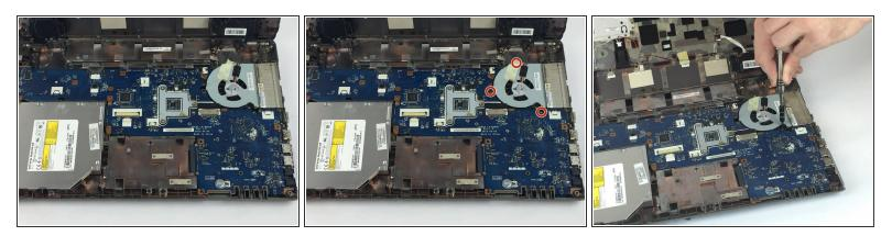
• Remove the three 3mm Phillips #0 screws from the fan.
