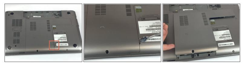
Use a plastic opening tool to lift up the cover and remove by hand.
