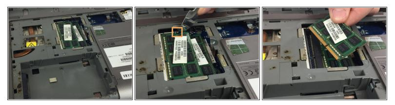
Two clips secure the RAM module in place, one on each side. Using your fingers, spread the clips away from the RAM module.
