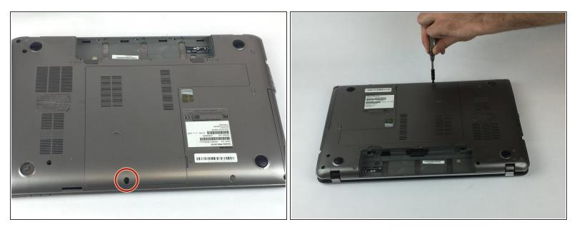
• Remove the 3mm Phillips #0 screw from the cover.
