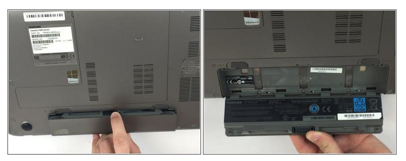
• Pull up on the battery to remove.
