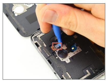
Remove the fingerprint sensor flex cable, using the plastic opening tool to lift it out.
