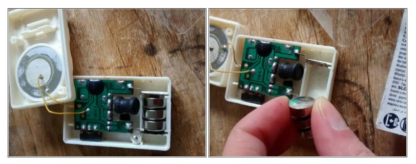
• Remove the batteries so you won't frighten yourself by a suddenly-working alarm (or break the alarm)
