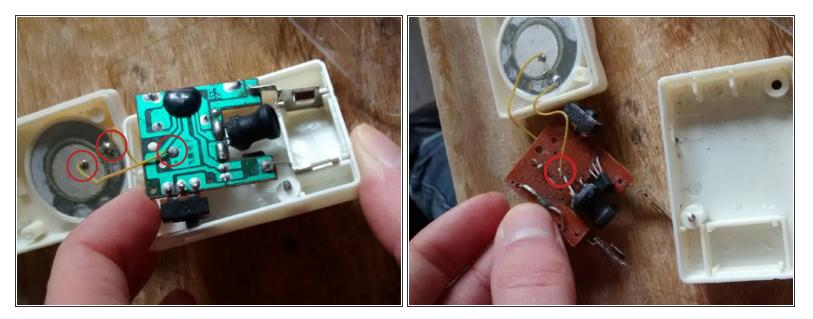
The wires weren't soldered good enough to make a sound. I applied a bit of fresh solder on the indicated places to make it work again
