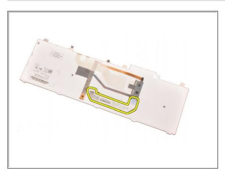
Peel the keyboard data cable away from the keyboard and remove.
