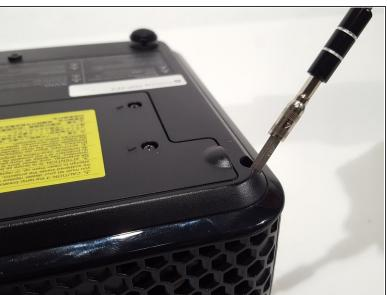
Start by removing the two screws on the bottom of the device as shown.
