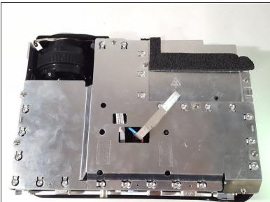
Unscrew the screws from the metal shielding to remove it.
